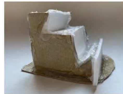
First prototype of the staircase mold which failed because the angled portions of the mold made the butter too thin
