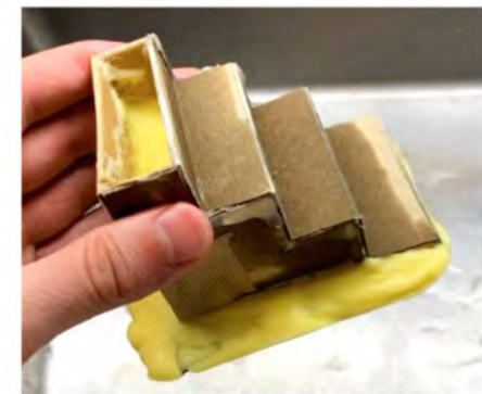
Liquid butter leaking from the cardboard mold sealed with hot glue
